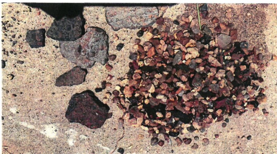
Figure 3: Flaked scale and gravel-pack filter material from the East well during baling on 15 June. The well video did not indicate any obvious breaks.
