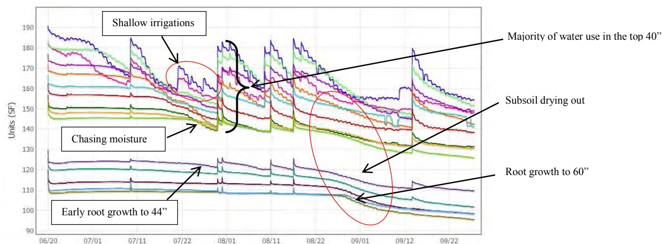
Figure 3. Krienke moisture graph (3 gpm)
