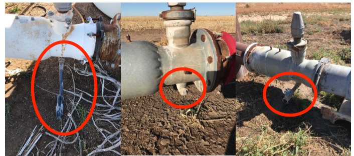
Noncompliant fixes outlined by the circles (left to right): LPD is Capped Off, LPD is missing and Plugged Off, LPD is Closed Off with a valve.
