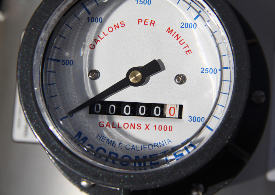
Pictured above is a McCrometer, with a totalizer read in gallons. All meters must be installed according to the manufacturer's recommendations. Broken meters must be reported to the district within 30 days and then replaced.
