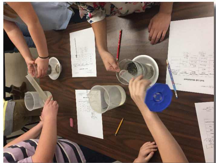
Students participate in a Soil Lab activity by measuring the water filtered through clay to see how porous the material is.
