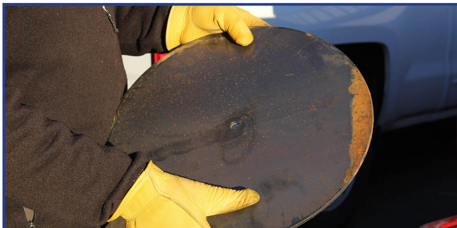
As part of the district’s open well-capping program, field staff carry 16-inch temporary caps to place over holes. The capping program reduces the risks of contamination of the aquifer and injury to people or animals.
