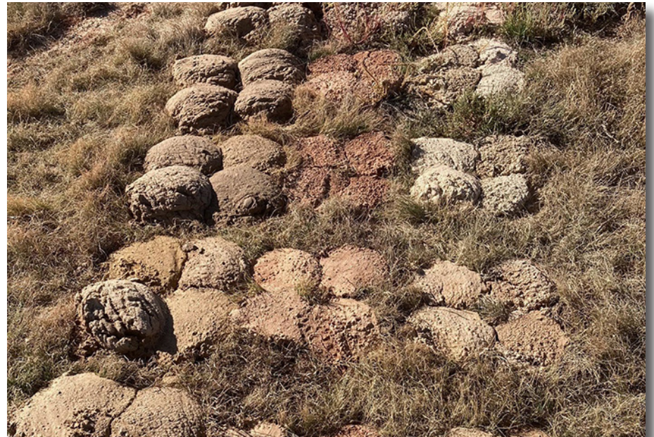
WCC test hole number 4 cuttings these help to understand the aquifer formation and the best location to drill a new well. Sand and Gravel produce more water and are indicators of a desirable well location.
