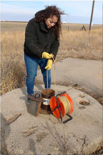
Natural Resource Specialist, Keila Davila is running an E-Line down a well to find the static water level of the well for Winter Water Levels.
