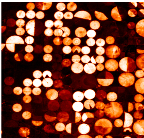
Satellite image generated by the Targeted Irrigation Management system to be used in both the “200-12” and “EPIC” demonstration projects. Vegetative index shows vegetation as the light areas on the image.
